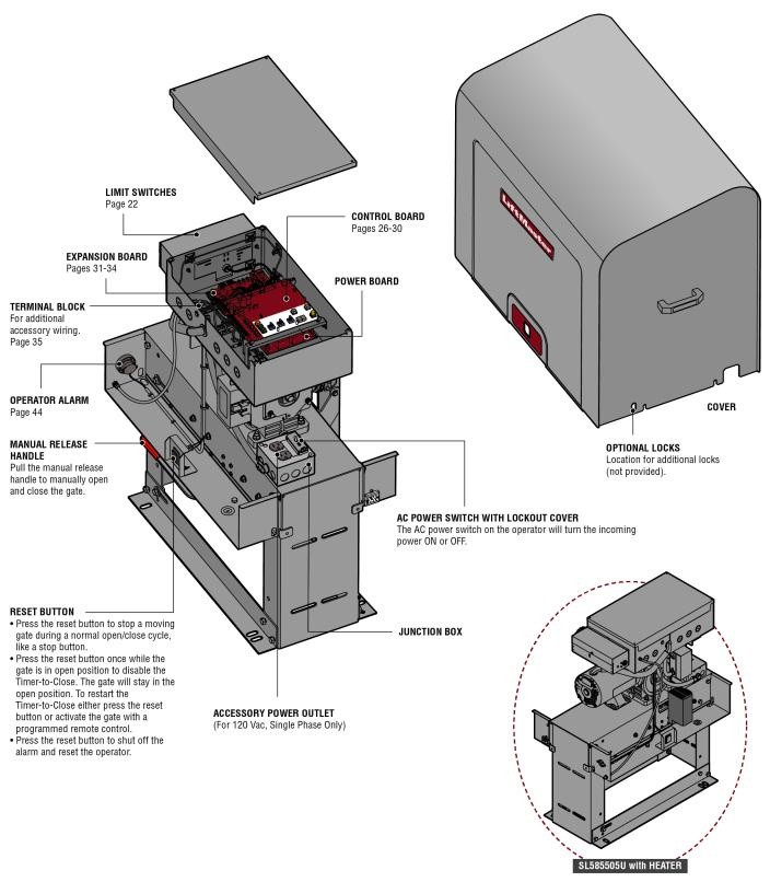
**NOTE:** The heater can only be turned off from the thermostat next to the heater.
