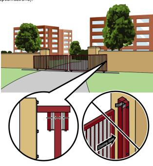
SAFETY CATCH ROLLERS Install catch rollers with safety covers on the side of a post or wall with a minimal distance of half an inch between the rollers and gate DO NOT use a gate catch post. Because the coasting distance may vary due to changes in temperature, it is NOT recommended to install a catch post in front of the gate's path. To do so will cause the gate to hit the post in certain instances.
