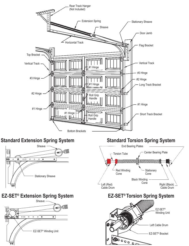
**NOTE:** The above illustration represents a composite of many of the features found on a variety of garage doors. While not representative of any one door, it provides a handy reference for the location of specific components.
